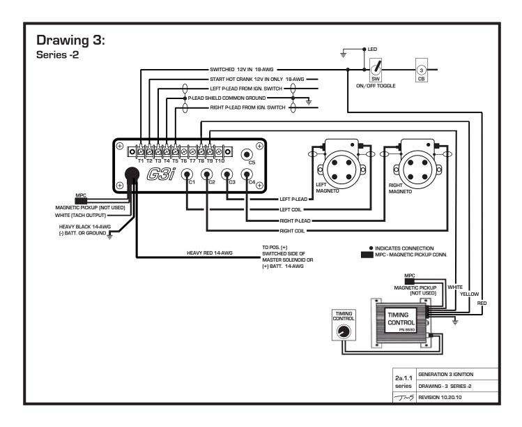
Left Magneto Normal Contacts are Trigger Source Left Magneto Lag – Retard Impulse Coupler MSD 8680 Adjustable Timing Control Timing Control Leads (Yellow - T8) (White - T9)
