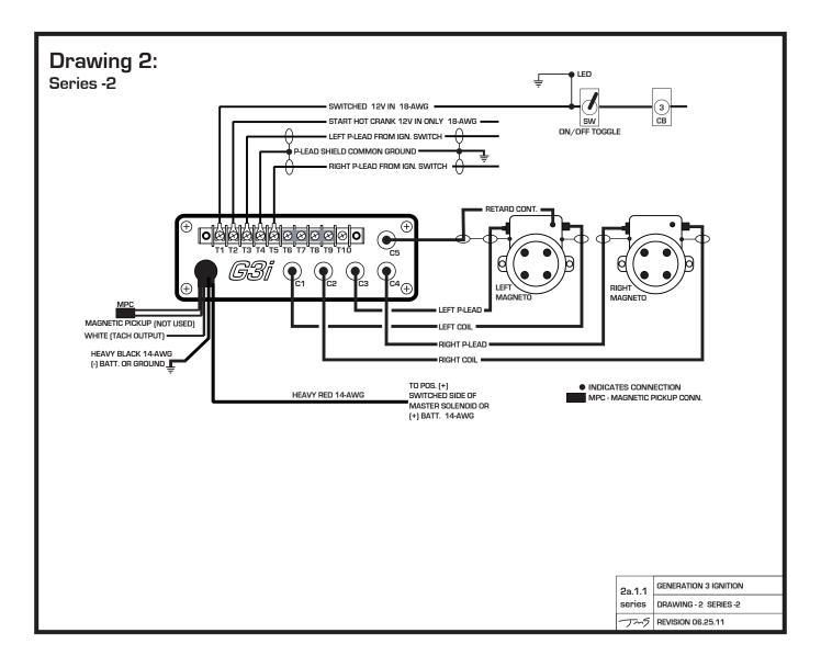
Left Magneto Normal Contacts are Trigger Source Left Magneto Retard Contacts / Active in Start \*\*\* BRIDGE TERMINALS (T6 - T7) (T8 - T9) \*\*\* Retard Contact P-Lead to BNC (C5)
