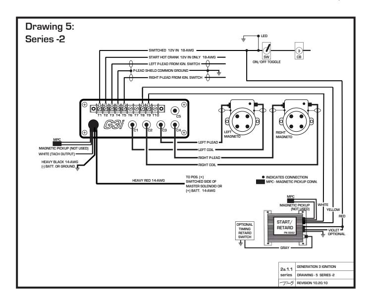
Left Magneto Normal Contacts are Start and Run Trigger Source With or Without Left Magneto Lag – Retard Impulse Coupler MSD 8982 Start/Retard Control Module Start/Retard Control Leads (Yellow - T8) (White - T9)
