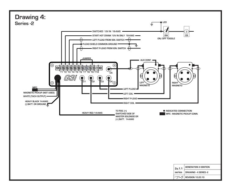
Left Magneto Auxiliary Contacts are Trigger Source
