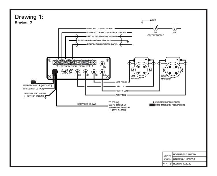
Left Magneto Normal Contacts are Trigger Source Left Magneto Lag - Retard Impulse Coupler \*\*\* BRIDGE TERMINALS (T8 - T9) \*\*\*
