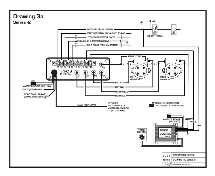
Left Magneto Normal Contacts are Trigger Source Left Magneto Retard Contacts / Active in Start MSD 8680 Adjustable Timing Control Timing Control Leads (White - T9) (Yellow - T10) \*\*\* BRIDGE TERMINALS (T6 - T7) \*\*\* Retard Contact P-Lead to BNC (C5)
