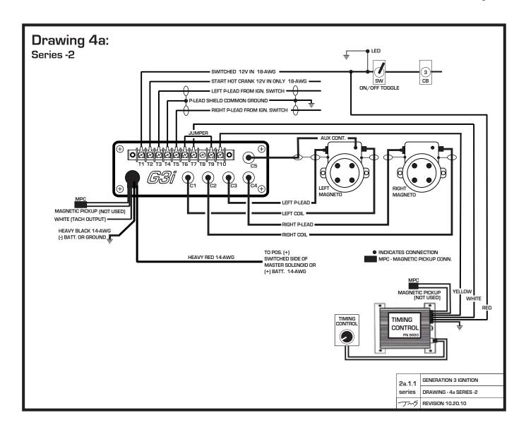
Left Magneto Auxiliary Contacts are Trigger Source Left Magneto Lag – Retard Impulse Coupler Starting on Normal Contacts MSD 8680 Adjustable Timing Control Timing Control Leads (White - T7) (Yellow - T10) Bridge terminals (T6 -T9) Auxiliary Contact P-Lead to BNC (C5)
